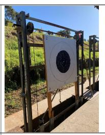
Target lowered showing scoring numbers located in each corner and wedges inserted to keep target stable in frame. Note dirt mound behind targets, watch there for shot impact.
