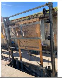
Rear view of target frame with target lowered showing counterweights and wires / pulleys (keep body away from moving parts). Never go behind target frame during an event.
